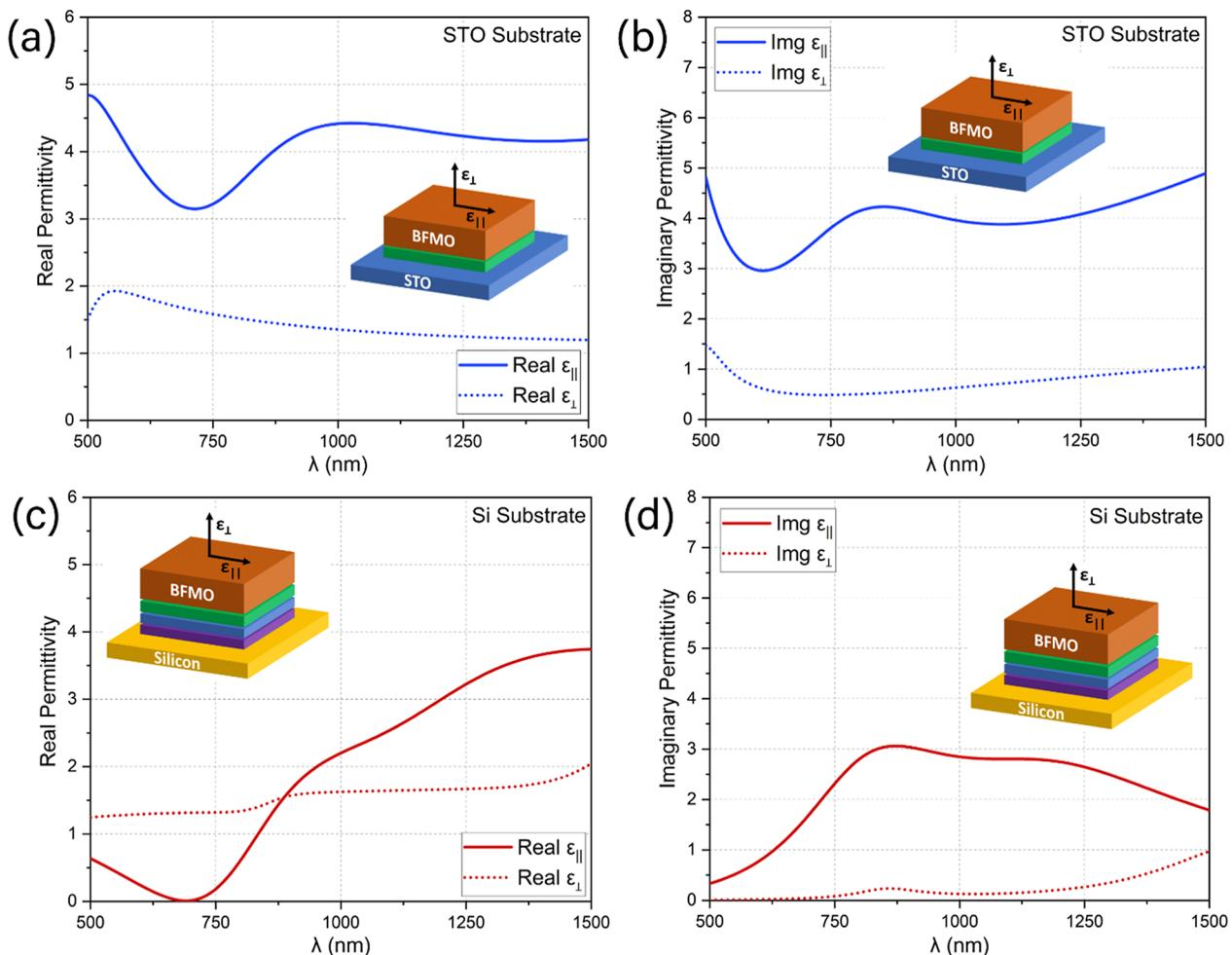
**Figure 5.** Optical characterization of the BFMO SC films. The (a) real and (b) imaginary permittivity for the film on the STO substrate. The (c) real and (d) imaginary permittivity for the film on the Si substrate.
