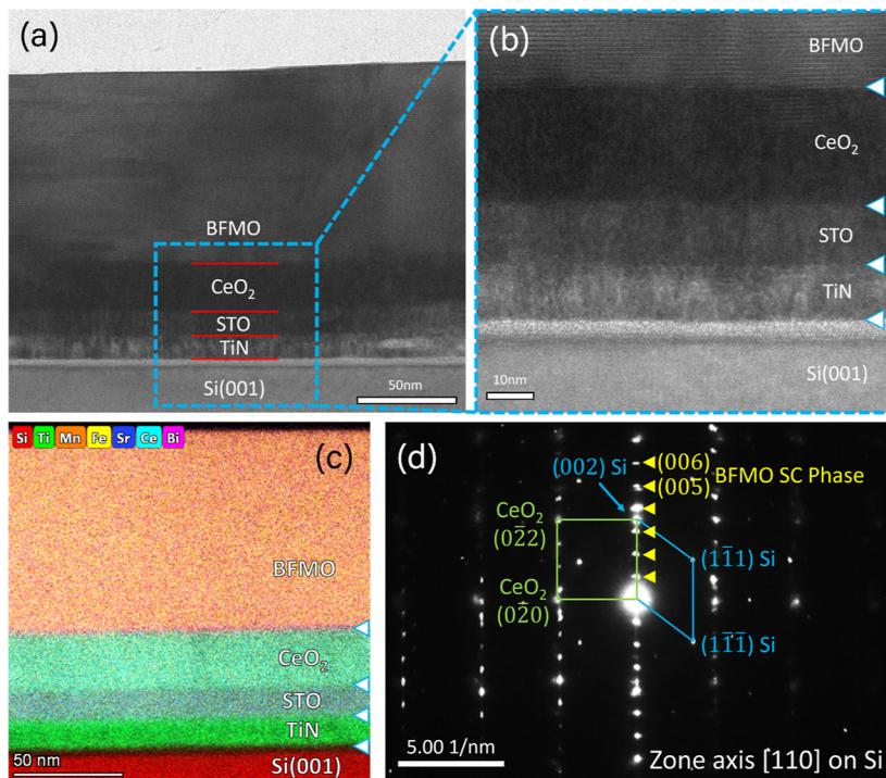
**Figure 2.** Microstructural characterization through TEM. (a) HR-TEM image of the layer stack on the Si substrate. (b) Higher magnification showing atomic-level epitaxy between layers. (c) EDS results confirming the composition of each layer. (d) SAED pattern showing epitaxial growth quality with expected orientation between layers.
