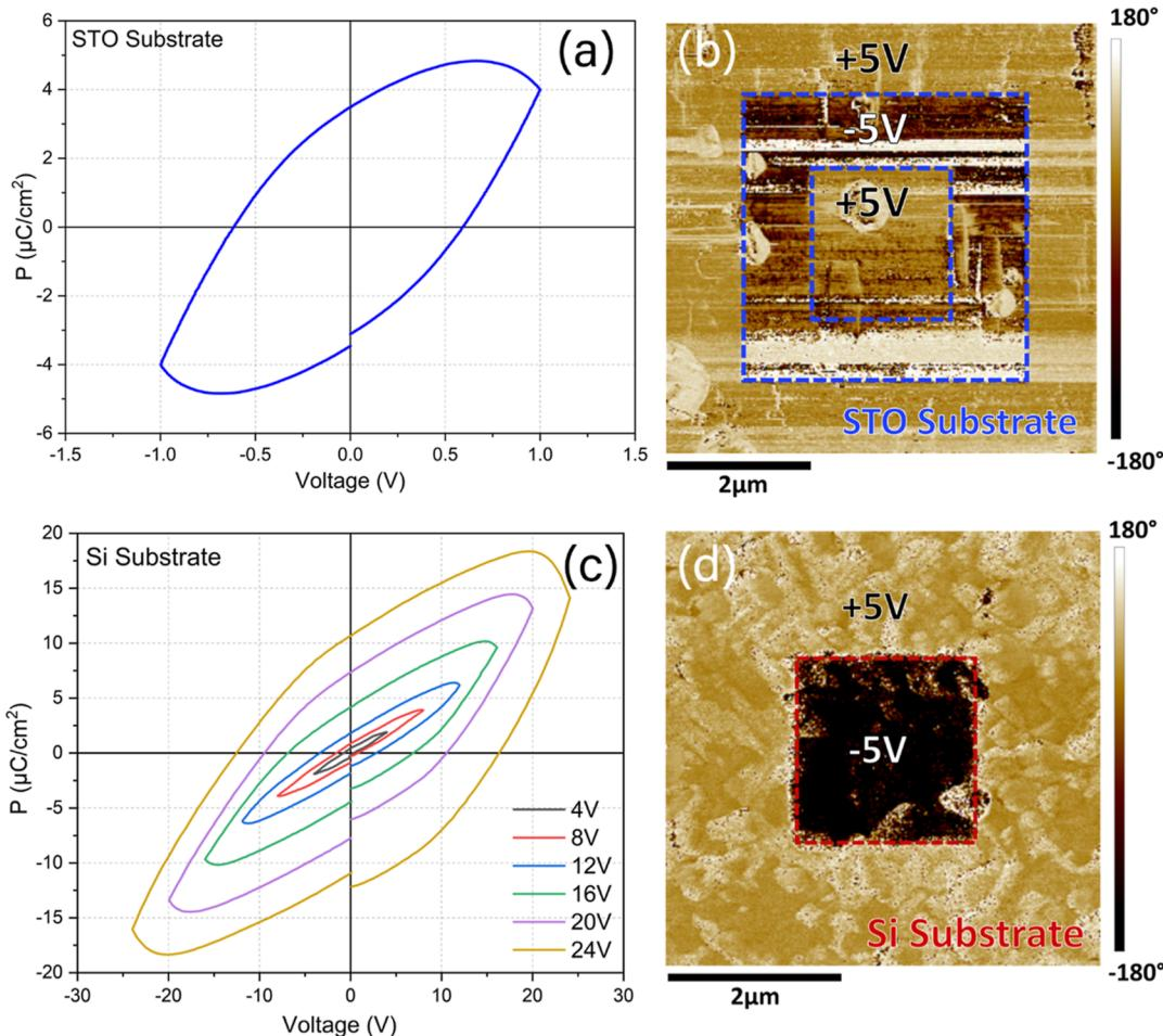
**Figure 4.** Electrical characterization of the BFMO SC film on (a,b) STO and (c,d) Si substrates. (a,c)  $P-E$  hysteresis loops allow for basic characterization of the ferroelectric properties of the film. (b,d) PFM phase maps show the ability of the film to hold the orientation of the polarization in a 2D area.
