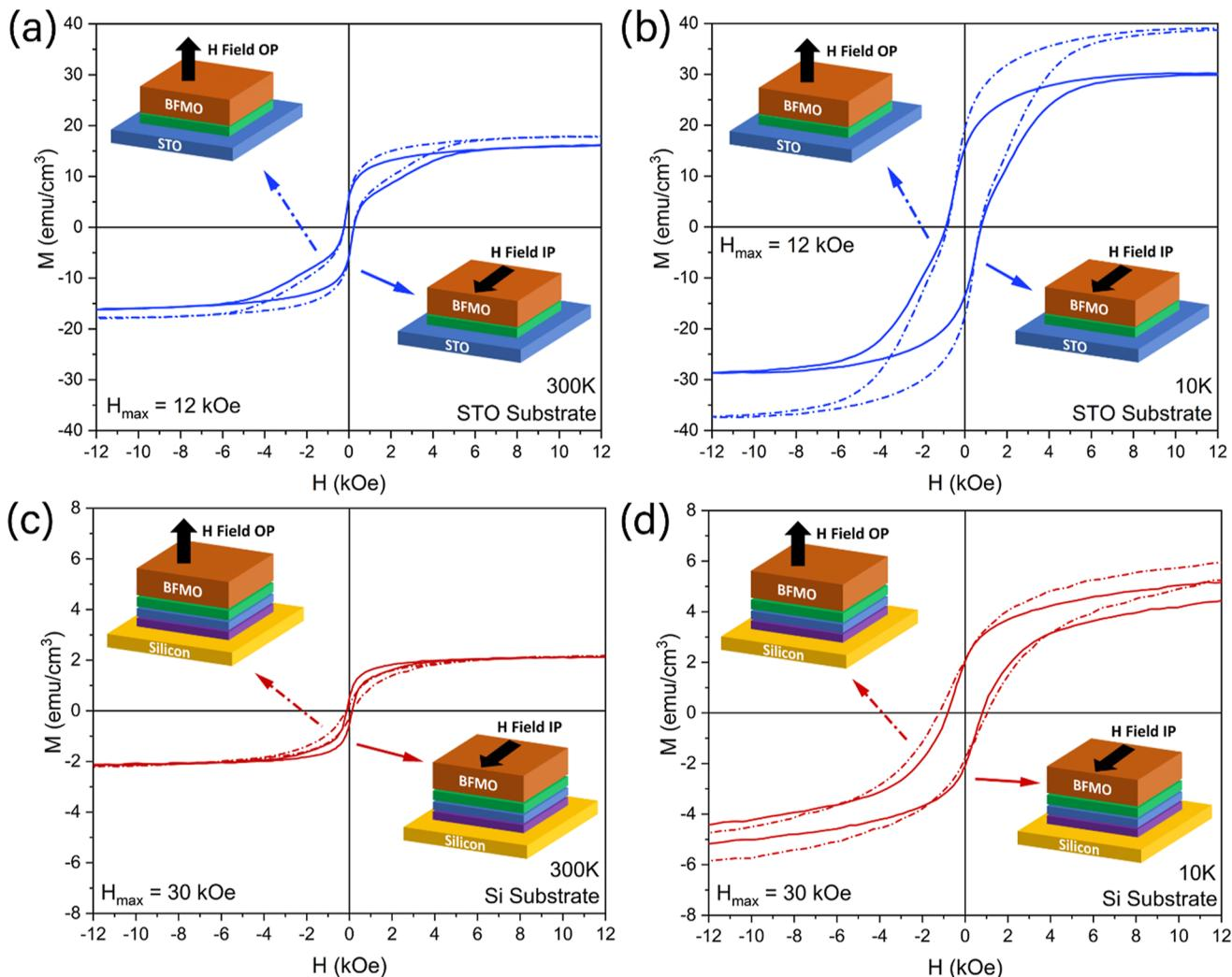
**Figure 3.** Magnetic characterization of the BFMO SC film on STO and Si substrates at temperatures of (a,c) 300 and (b,d) 10 K. The plotted field range is selected to highlight coercivity and remanence, while the actual maximum applied field to ensure saturation is listed in each case.
