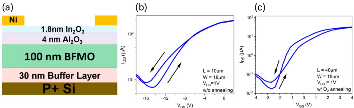
**Figure 6.** Device testing of the FeFET. The (a) schematic and the output transfer characteristics (b) before and (c) after O<sub>2</sub> annealing.
